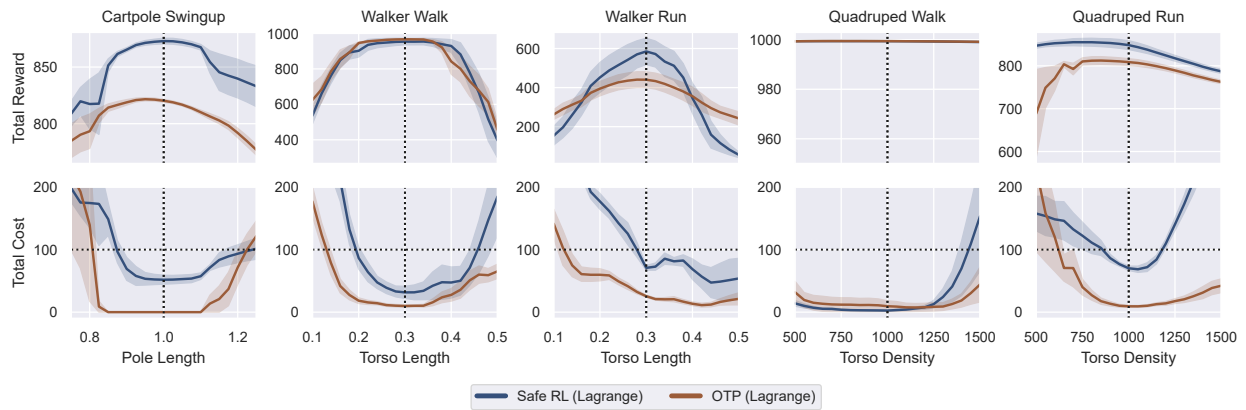
Figure 10: Comparison of OTP with standard safe RL across tasks and test environments using a Lagrangian-based update method. Shading denotes one standard error across policies. Vertical dotted lines represent nominal training environment. Top: Total reward. Bottom: Total cost, where horizontal dotted lines represent the safety budget and values below these lines represent safety constraint satisfaction.
