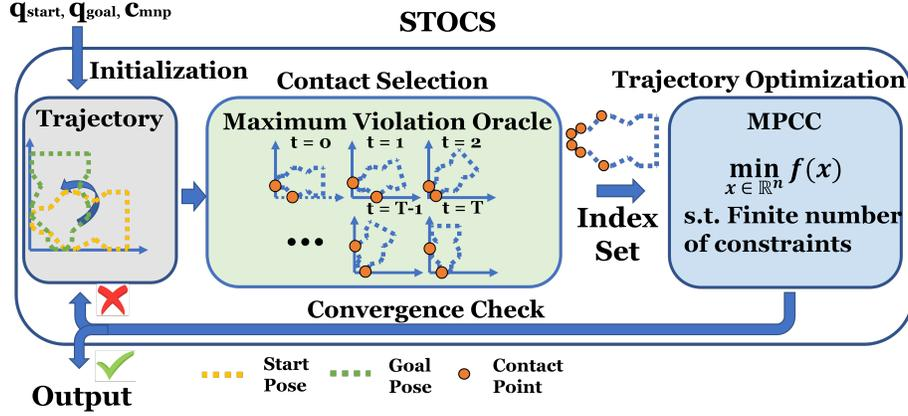
Fig. 4: Illustrating the workflow of STOCS. Given the start pose  $q_{start}$ , goal pose  $q_{goal}$ , and a manipulator contact state  $c_{mnp}$ , STOCS iterates between using the Maximum Violation Oracle to instantiate contact points, and solving a finite dimensional MPCC to decide a step direction until the convergence criteria is met. STOCS does not need a predefined contact set and can select the contact points simultaneously while solving trajectory optimization. [Best viewed in color.]
