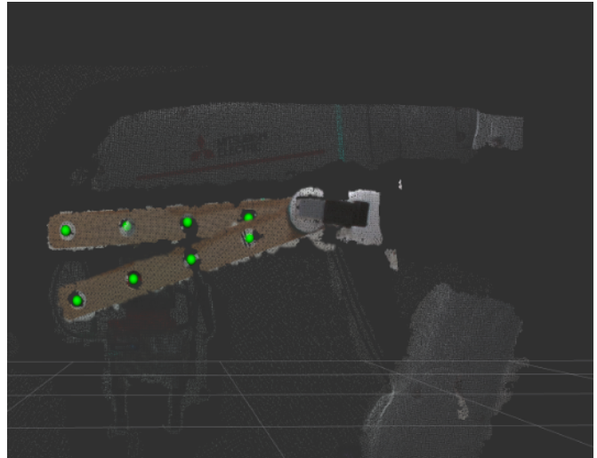
Fig. 9: In this figure, we show the range of the placement of the bar in the stationary gripper for which the vision algorithm is able to detect the location of all the four holes.
