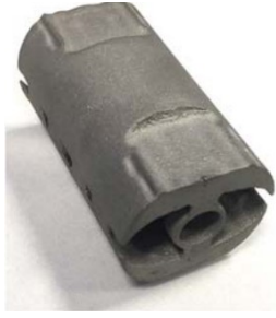
Fig. 4. BESO optimized rotor fabricated using SLM technique in [10].
