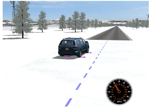
Fig. 2. Illustration of a vehicle performing lane-change maneuvers in CarSim, while friction parameters and uncertainty are adapted online for SNMPC. The purple arrows show the lateral forces acting onto the wheels.
