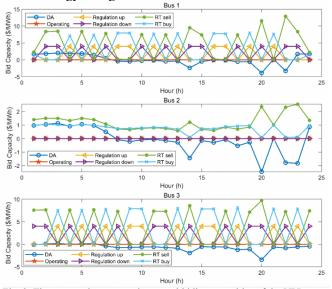
Fig. 3. The expected energy and reserve bidding capacities of the VPP
