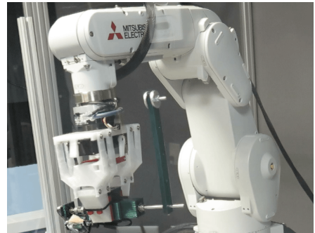
Fig. 5: The Furuta Pendulum (3D printed in color green) held in the gripper at the swing-up position reached using the learned controller.
