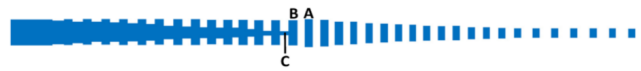
Fig. 17. Schematic of a SOI edge coupler based on SWG [64] (Copyright in 2015, OSA).
