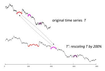
Fig. 10. top) The original time series. bottom) Rescaling the original time series by 200%. The first (red) pattern in the original time series matches very well with the second (pink) pattern in the rescaled time series.
