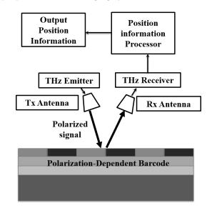
Figure 1. The diagram of proposed THz encoder system.
