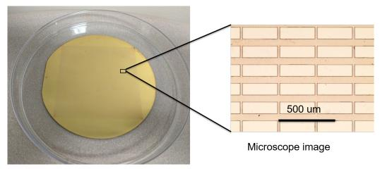
Figure 5. A picture of fabricated metamaterial absorber sample.
