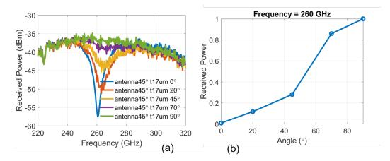
Figure 6. (a) Experimentally measured reflection spectrum for different rotation angles of the metamaterial absorber sample. (b) The reflection as a function of rotation angle at the resonant frequency of 260 GHz.
