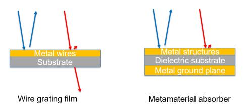
Figure 2. (a) The response of a wire grating film polarizer to two different polarization. (b) The response of a polarizationdependent metamaterial absorber to two different polarizations.
