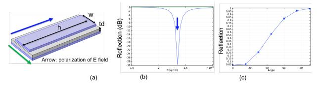
Figure 3. (a) The unit cell structure used for simulation: The top metal (gold) patch has width  $w = 120\mu$ m and length  $h = 340\mu$ m, and the unit cell size is  $175\mu$ m  $\times 350\mu$ m. The thickness of the dielectric spacer (parylene-C) is  $t_d = 17\mu$ m. The metal layer thickness is 100 nm. (b)Simulated reflection spectrum with two different polarizations. (c) Reflected power as a function of rotation angle.
