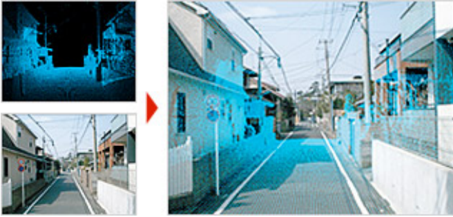
Fig. 2 Map creation where images are projected by superimposing laser point cloud data onto camera images
