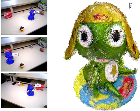
Figure 5. Reconstruction results on example scene 2, where we model an object which consists of mostly non-planar segments: example keyframes from the sequence (left), reconstructed point cloud (right).
