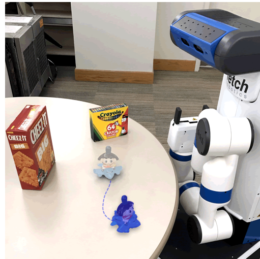
Figure 1. Illustrative representation of the system. The mobile robot used in the experiments detects a moving object and generates an object map separately from a static map corresponding to the static environment.
