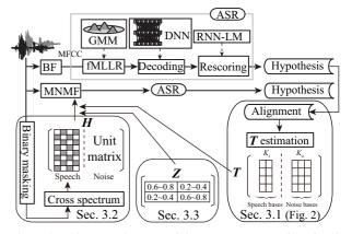
Figure 3: Schematic diagram of the ASR system combined with the proposed initialization methods.
