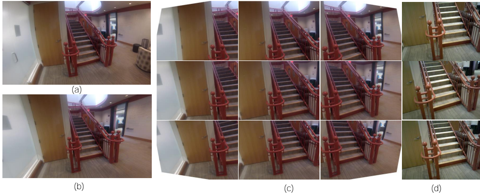
Fig. 4. (a) The original wide-angle monocular image. Straight lines in the scene are distorted due to the fisheye lens distortions. (b) A single undistorted monocular image generated to cover the entire FOV of the original image. Although the straight lines remain straight, the peripheral regions are stretched compared to the central regions due to the perspective distortions, resulting in different feature descriptors in different regions. (c) Nine virtual monocular images generated to cover the entire FOV of the original image. (d) Example RGBD images of the same scene, whose appearance is similar to the virtual images (c) compared to the single undistorted image (b).
