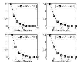
Fig. 2. The comparison of  $P_{ik}$  at kth iteration of ith subsystem and their optimal values
