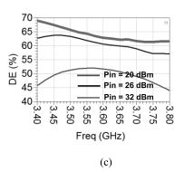
Fig. 5: Large-signal simulation results of proposed wideband Doherty PA (a) output power versus drain efficiency (DE), (b) gain response at 3.4-3.8 GHz, (c) drain efficiency across 3.4-3.8 GHz for various conditions of input power.
