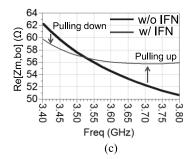
Fig. 4: (a) S-parameter simulation results, (b) real part of  $Z_m$  both at back-off an peak input power, (c) frequency response of real part of  $Z_m$  at back-off with and without impedance flattening network across 3.4-3.8 GHz.
