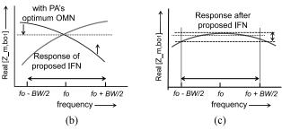
Fig. 2: Block diagram of (a) proposed impedance flattening network (IFN), (b) frequency responses of PA's optimum output matching network in typical condition and proposed IFN alone, (c) resultant frequency response after incorporating the IFN in load modulation network.
