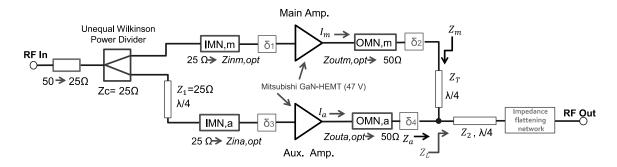
Fig. 3: Complete block diagram of the proposed wideband Doherty power amplifier with impedance flattening network.
