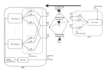
Fig. 1: Simplified architecture of the transmitter and receiver in uplink communications, where  $\beta_l$  denotes the gain of the lth scattering cluster.
