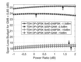
Fig. 5: Span loss budget for the 2A8PSK-based and the conventional TDH at 4.5 bits/symbol, as a function of power ratio, at the nonlinear and linear regions. The arrows indicate the optimum power ratio
