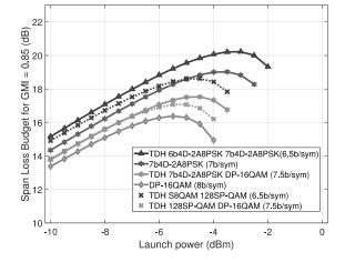
Fig. 2: Span loss budget for various modulation formats in the range of 4 - 6 bits/symbol.
