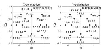
Fig. 1: Constellation and bit-to-symbol mapping of 2A8PSK [10].
