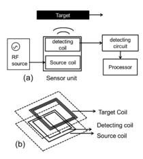
Fig. 2. (a) Block diagram of the proposed sensing system. (b) Example design of sensor structures.
