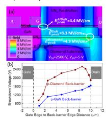
Fig. 4. (a) Simulated electric field distribution in GaN-on-diamond HEMTs with a patterned p-diamond back-barrier, at the bias of  $V_{GS}$ =-5 V and  $V_{DS}$ =2500 V. The gate edge to back-barrier edge distance is 8.5 µm. (b) Dependence of device breakdown voltage on the gate edge to back-barrier edge distance for GaN HEMTs with p-diamond and p-GaN back-barriers. The geometry and doping of p-GaN and p-diamond back-barrier are extracted from Fig. 3 (f) for a charge balance condition with 2DEG.
