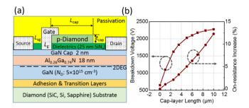
Fig. 8. (a) Schematic structure of the GaN HEMTs with a p-diamond cap-layer. The  $L_{sg}$ ,  $L_g$  and  $L_{gd}$  are set as 1.5 µm, 2 µm and 10 µm. (b) Dependence of BV and  $\Delta R_{on}$  as a function of cap-layer length  $L_{cap}$ . The cap-layer thickness  $t_{cap}$  and doping level are 60 nm and  $1 \times 10^{18}$  cm<sup>-3</sup>.
