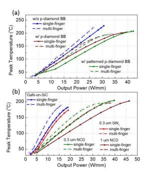
Fig. 6. Simulated peak temperature dependence on output power density for (a) GaN-on-diamond HEMTs with and without a p-diamond back-barrier (BB) and with an optimized patterned p-diamond BB; (b) GaN-on-SiC HEMTs with 0.3  $\mu$ m SiN<sub>x</sub> passivation, and GaN-on-diamond HEMTs with 0.3  $\mu$ m SiN<sub>x</sub>, 0.3  $\mu$ m NCD and 1  $\mu$ m NCD passivation. Single-finger and multi-finger simulation for all devices are conducted.
