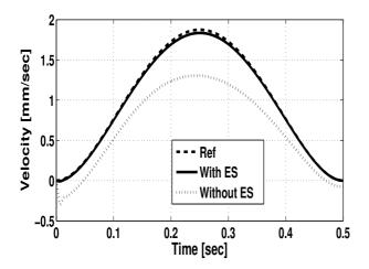
Fig. 2. Obtained Armature Velocity vs. Reference Trajectory
