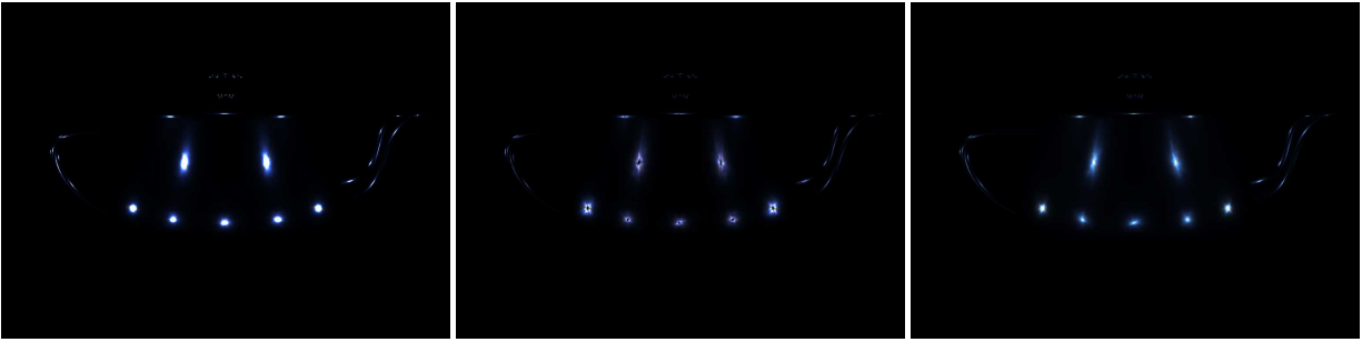
Figure 9: Nonlinear spaces generate valid BRDFs where linear spaces fail. Original BRDF corresponding to a point A on a 45 dimensional hyperplane (left). Physically implausible reflectance (hole in the middle of the specular highlight) corresponding to moving away from a point A on the 45 dimensional linear subspace (center). Physically plausible reflectance corresponding to moving equally far away from point A on the 15 dimensional non-linear manifold (right).
