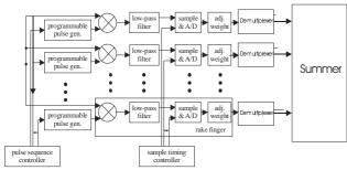
Figure 3 Rake receiver structure
