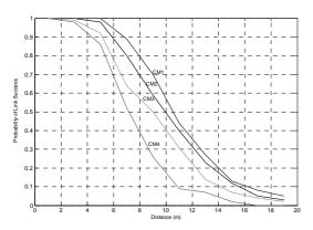
Figure 4 Probability of link success as function of distance for 110Mbit/s mode
