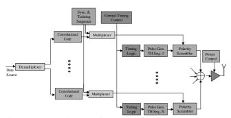
Figure 1 Block diagram of the transmitter
